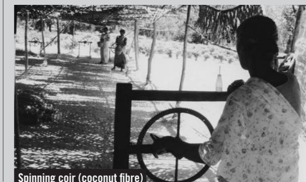
Spinning coir (coconut fibre)
